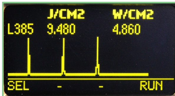
Graph View showing data collected on three LEDs
