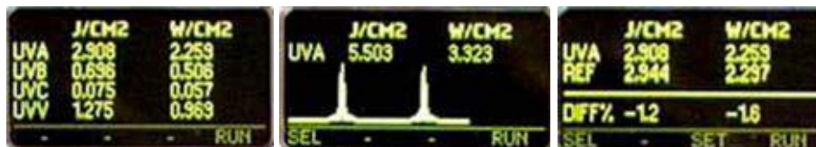
Left to Right: Data Screen Mode, Graph Screen Mode and Reference Mode from UV Power Puck® II and UVICURE® Plus II screens
