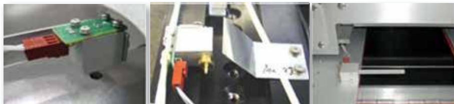
Examples of Compact Sensor Mounting Locations Left to Right: Mounted behind the reflector looking at bulb, mounted behind reflector looking at reflected UV, mounted near cure surface and using quartz rod to pick up UV
