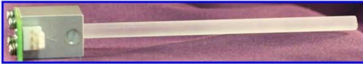
Top Left: Compact Sensor with Quartz Rod installed
